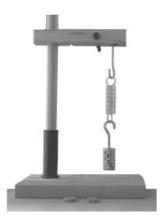
She uses a ruler to measure the vertical distance h between the bottom of the mass hanger and the base of the stand.
